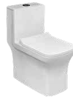
META SOPMETWPP3025 Washdown Flushing PP Soft Close Seat Cover Size: 645 mm x 360 mm x 725 mm S-Trap: 225 mm
